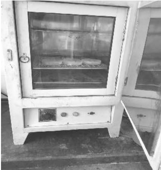
Specimens Stored in Artificial Saliva at 37 Degree Celcius in Incubator in 100% Relative
